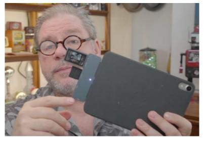
A third method for importing would be to use a USB hub. This plugs into your iPad on one end via USB C and the other side has multiple connection options. You can insert the SD card into one slot and a separate hard drive into another slot.
